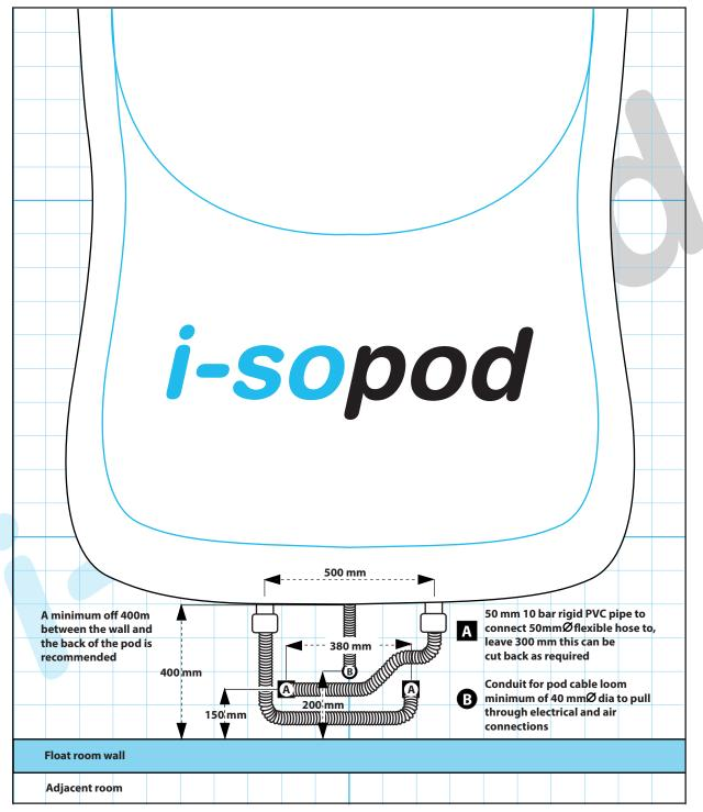
• Note: Flexible hoses are routed as above due to the bend radius of the PVC hose.
